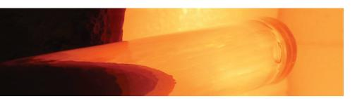
ROD MOULDING of Glass is a specialist process employing the use of Polished rods of Glass which are heated until they become soft and then offered into an accurate tool, forming a chill free FIRE POLISHED component.
